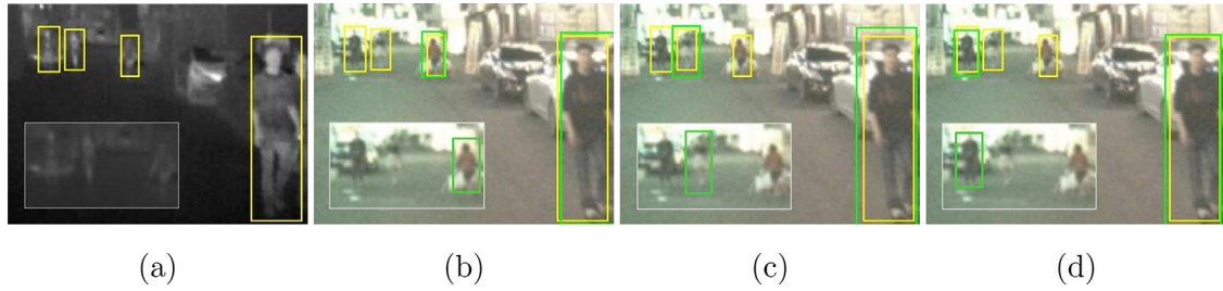
Fig. 1. Examples of complementary detection results using convolutional features from only color, thermal, and color-thermal fusion channels. Boxes with yellow and green color represent ground-truth and estimated bounding boxes, respectively. With a thermal image in (a), the pedestrian candidates are detected using individually learned features on (b) the color image only, (c) the thermal image only, and (d) the existing fusion feature [18] on both color and thermal images. The existing fusion method [18] cannot fully reveal the complementary potential between color and thermal images, but rather individually learned features on each modality can produce reliable performances in some circumstances. By synergistically fusing these features, our system can maximize the pedestrian detection performance under all challenging circumstances. (For interpretation of the references to color in this figure legend, the reader is referred to the web version of this article.)
