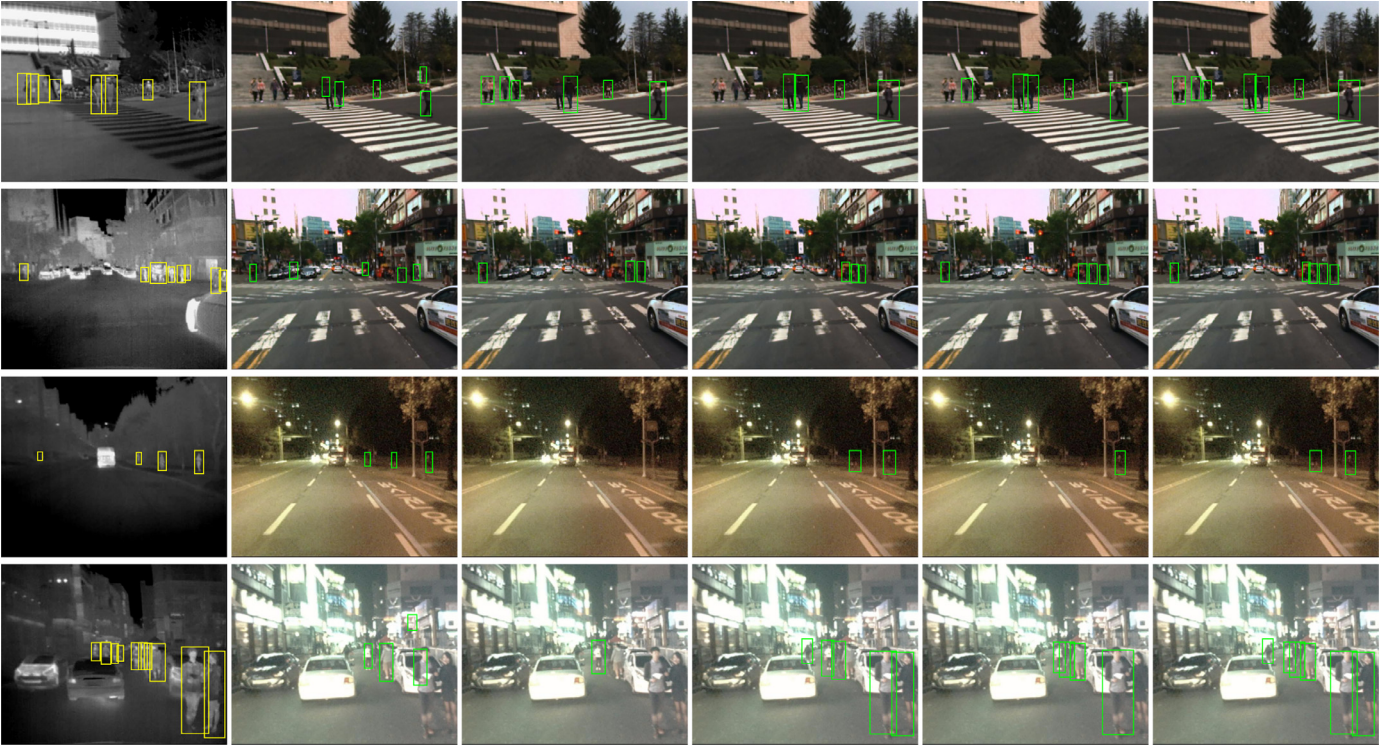
Fig. 8. Qualitative comparisons of detection results on the test set of KAIST multi-spectral dataset [20]. (From left to right) Thermal images with ground-truth, detection results from Choi et al. [19], Faster R-CNN [12] with color and thermal channels, half-way fusion [18], and the proposed method.
