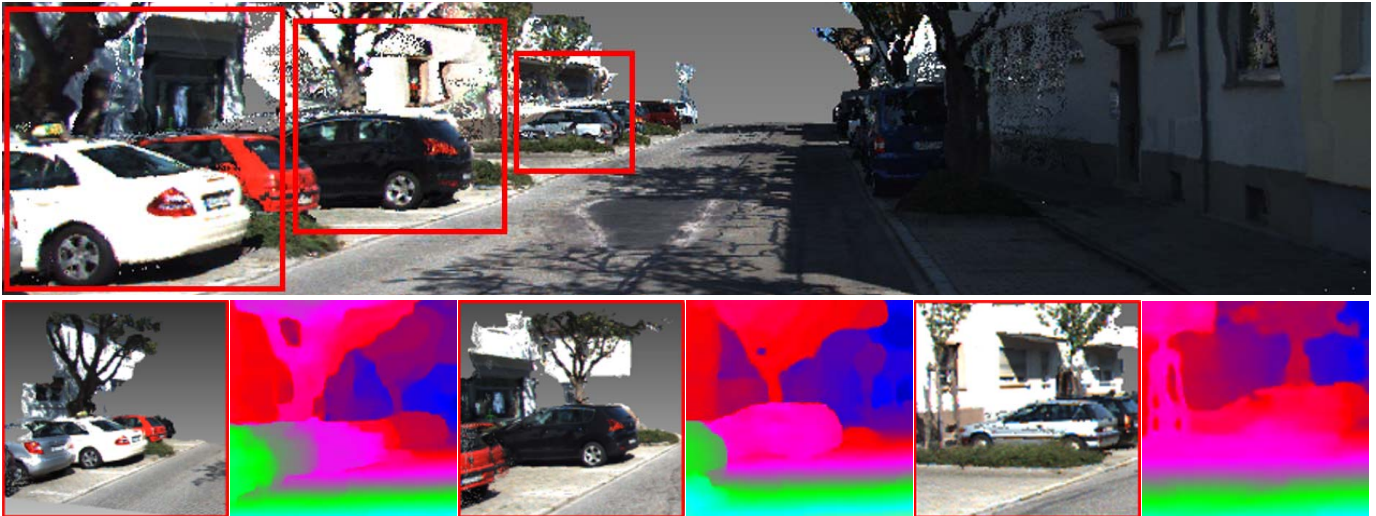
Fig. 13. Examples of outdoor 3D scene reconstruction using proposed method on KITTI dataset [19]. By leveraging complementary properties of LiDAR and stereo data, we can successfully reconstruct 3D model even in challenging outdoor conditions.
