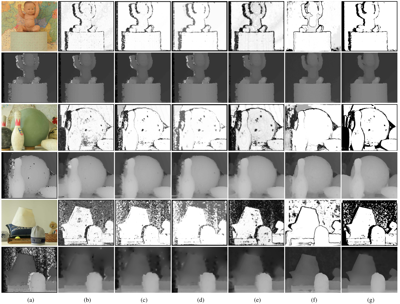
Fig. 12. The confidence and refined disparity maps on MID 2006 dataset [39] using MC-CNN+mod. (1st and 2nd rows), +GCPs (3rd and 4th rows), and +AGCPs (5th and 6th rows) (a) Color images and initial disparity maps, refined disparity maps with confidence maps estimated by (b) Haeusler et al. [23], (c) Poggi et al. [29], (d) Seki and Pollefeys [28], (e) proposed wo/CVR [41], (f) proposed, and (g) ground truth confidence map.
